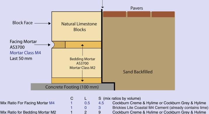
Note: Only use clean damp bricklaying sand. Final mortar colour will depend on mix ratio and the sand colour.
