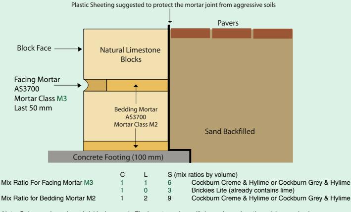
Note: Only use clean damp bricklaying sand. Final mortar colour will depend on mix ratio and the sand colour.
