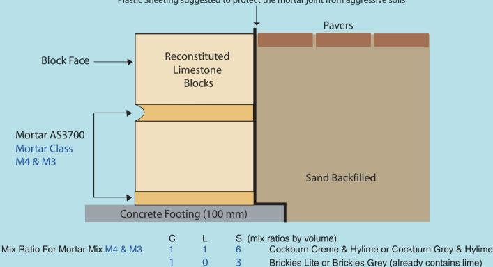
Plastic Sheeting suggested to protect the mortar joint from aggressive soils
